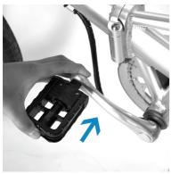
**Pedals** press pedal inward and push upwards, to unfold just pull it to original position
