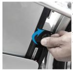
Turn the key to the 'ON' position. A red LED will illuminate below the key socket. If the light flashes, read the **Troubleshooting** section of this manual. If it shines steadily, you're ready for the next step.
